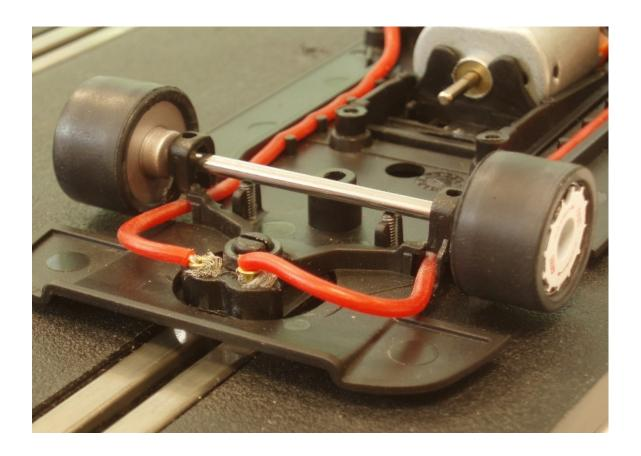
The 6 mm long hexagonal screws must be inserted in the holes and their position adjusted to raise the axle to the desired position:
