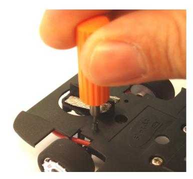
The upper loop that retains the axle has two holes. They are designed to 'clip' the front bushing in place, but accept hexagonal M2 grub screws (usually 3 mm long). The position, and vertical run, of the front axle can be controlled by adjusting the position of these screws.
