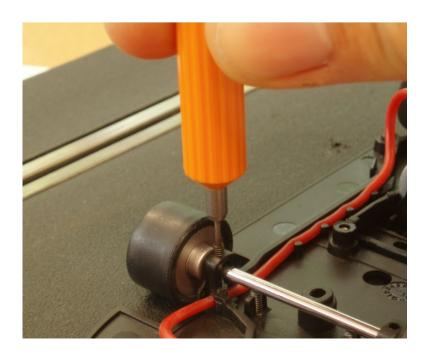
The upper loop is designed to accept a metal bushing like the ones used for the rear axle, if so desired:
